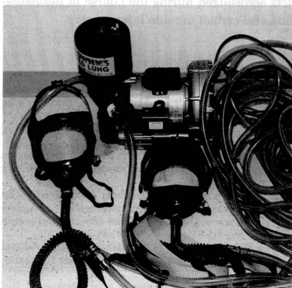
Fig 1. The air compression unit, two masks, and two segments of 15 m (for each mask) of hose.
