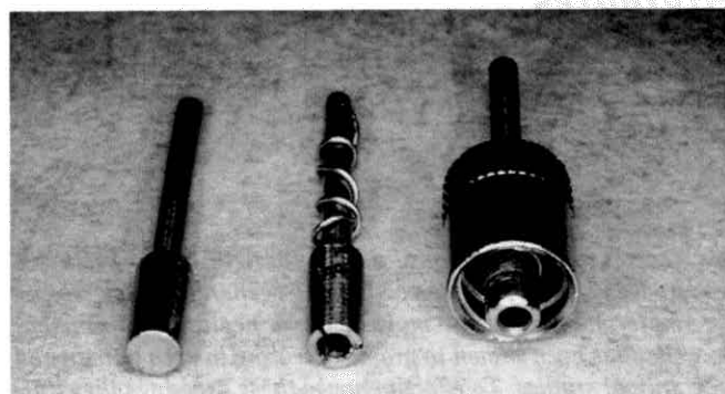
Figure 1. Electrosurgical adapters on frontal view. The central modified electrosurgical adapter is flanked by the larger Luer-lok adapter (right) and the original solid-steel traditional adapter (left).
